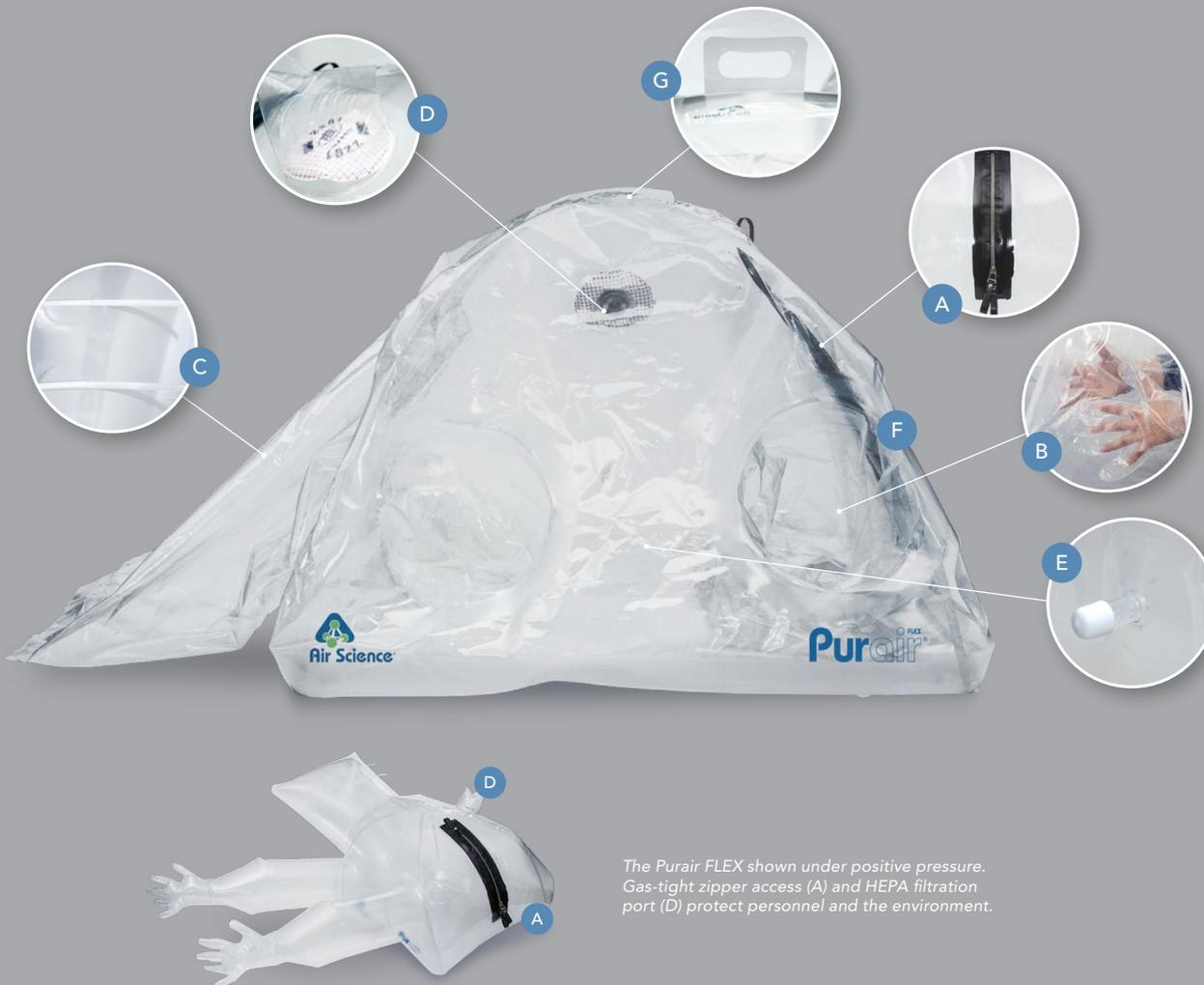
The Purair FLEX shown under positive pressure. Gas-tight zipper access (A) and HEPA filtration port (D) protect personnel and the environment.
