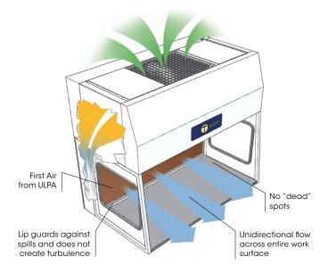
The Air Science Horizontal Laminar Flow cabinet provides unidirectional airflow directly from the ULPA filter across the entire work surface. Cabinet design ensures no air dead spots to interfere with first air delivery and a rear lip on the work surface guards against contamination from spills.
