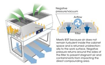
In the Air Science Vertical Laminar Flow cabinet, first air contacts the work surface directly as it flows from the ULPA filter. The VLF incorporates a perforated rear panel to combat turbulent or stagnant air in this area of the work zone. Additionally, no stagnant air exists on the ceiling of the unit as perforations in the ceiling panel to the side of the filter gasket help create an area of negative pressure to ensure all air entering the work zone is ULPA-filtered first.
