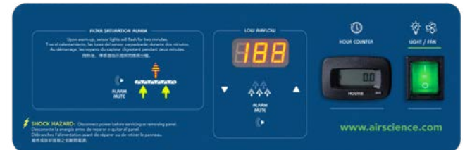
FSA/AutoCAL Control Panel
