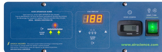
FSA/Autocal Control Panel
