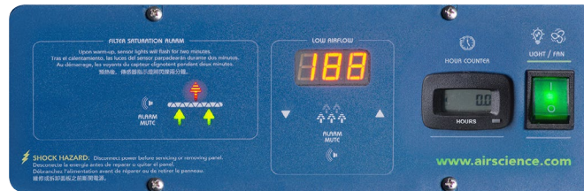
FSA/Autocal Control Panel
