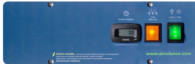
Basic Control Panel
