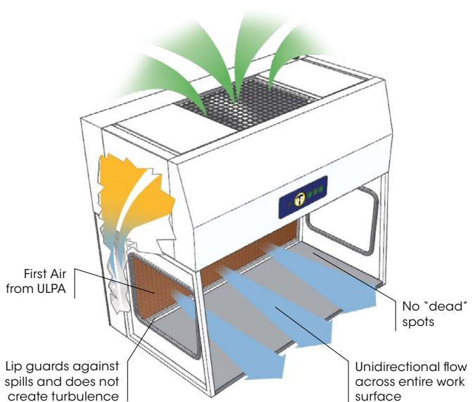
*The Air Science Horizontal Laminar Flow cabinet provides unidirectional airflow directly from the ULPA filter across the entire work surface. Cabinet design ensures no air dead spots to interfere with first air delivery and a rear lip on the work surface guards against contamination from spills.*
